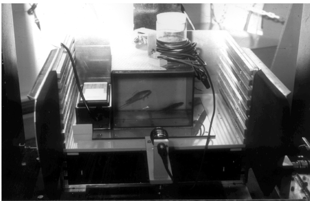
Fig. 1. The experimental set-up showing the aquarium bolted to the turntable. The video camera at the front, the light source at the top and the closed tube used for filling the aquarium are clearly visible.
